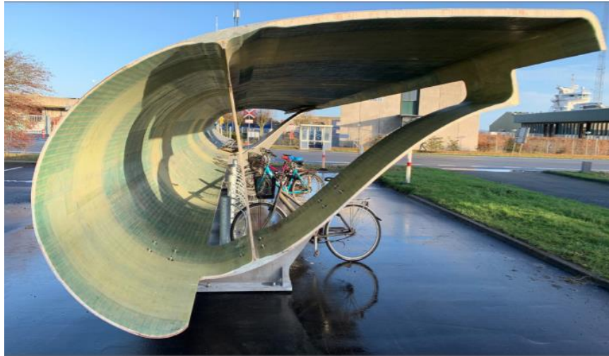
Figure 7: Repurposing wind turbine blades as a bike shed in Denmark 5
